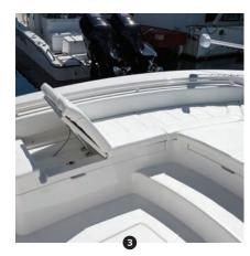
① A hydraulic jack plate and Power-Pole shallow-water anchor are among the desirable options. ② The dash affords plenty of room for electronics, gauges, stereo and more. ③ Port and starboard seats bookend the forward casting deck. Foldaway backrests turn them into loungers.
